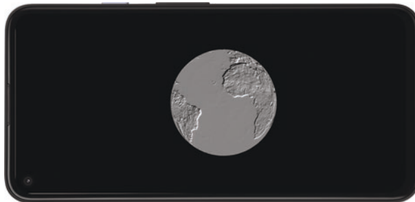
Figure 15-12. Output of the emboss shader applied to a sphere
