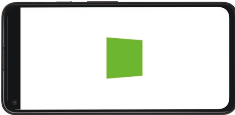
Figure 15-3. Output of the shader in Listing 15-4, with constant fragment color
