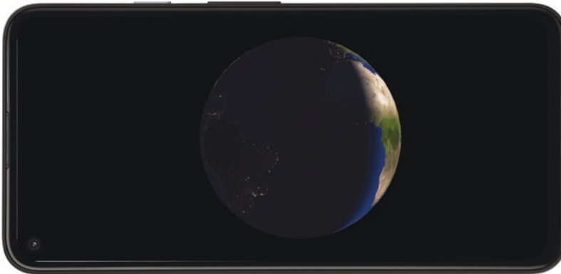
Figure 15-16. Interpolation between day and night Earth maps using the azimuth angle
